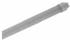
imag-20W-T8-4FT(I004) 20w =36W, BALASTRO 1.7G, 1900LUMS, +/-10%, 5500k - 6500k, 1200. LONG, 30Ø, Blanco mate
