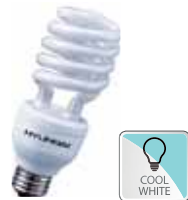
HYPSS-3227CW (H156) Half spiral E27 32W 4200K, 220-240V, 50/60HZ, 2052LM, 8000H 185LONG, 70Ø
